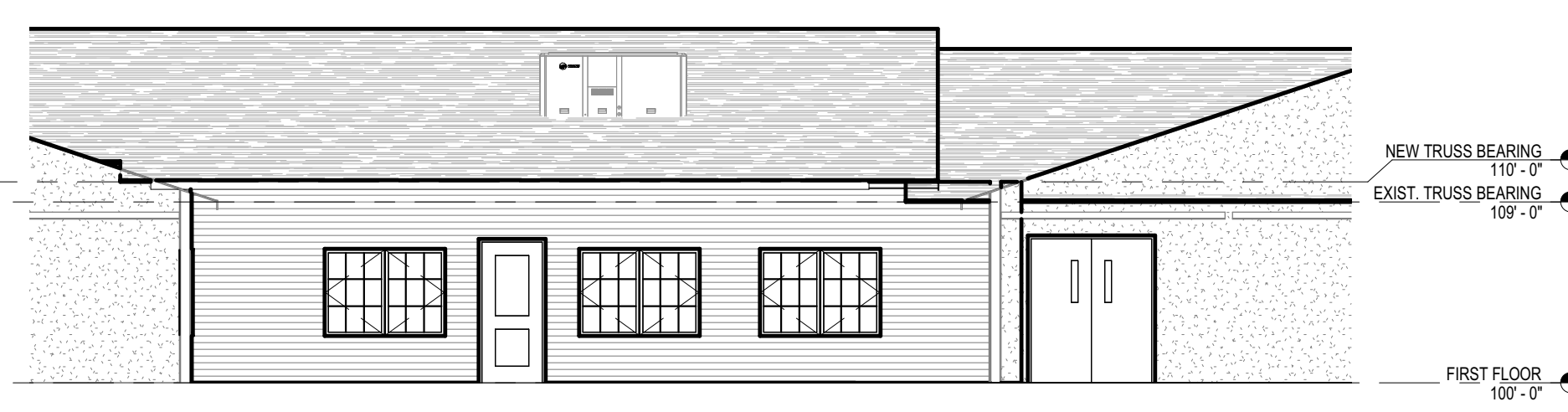
7 UNIT 'C' WEST ELEVATION - SOUTH A4.01 1/8" = 1'-0"
